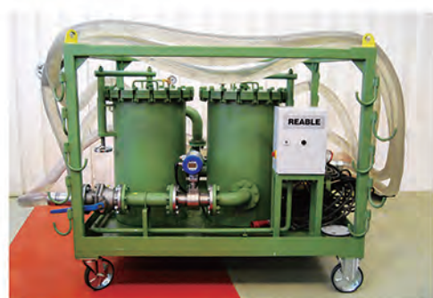
油冲洗设备 Oil washing equipment
